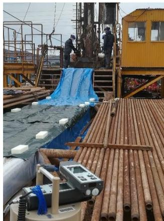
*Preparation for the rescue of the well-logging geophysical probe*
